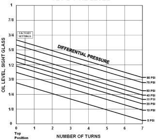
Note: Data obtained using POE lubricant at 86°F with a 1 inch diameter sight glass.
