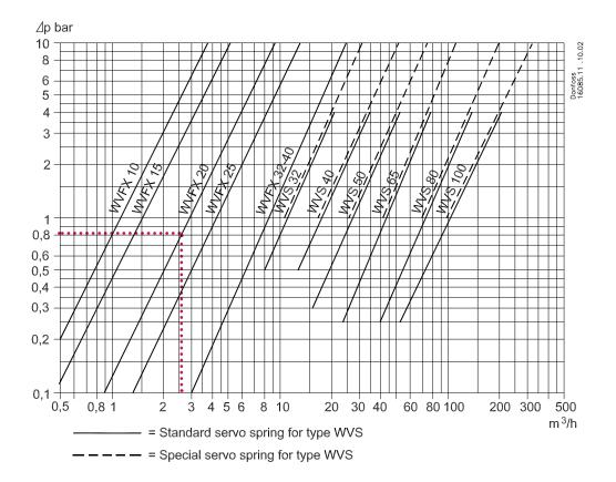
Selecting WVFX 20 Code number The saturated pressure for R404A  $T^c = 35^{\circ}C \Rightarrow P_c = 15.5$  barg
