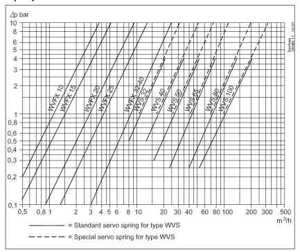
The capacity curves show the capacities of individual valves (water quantity in m<sup>3</sup>/h) depending on the pressure drop across valves.
