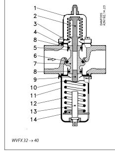
The valve cone (7) is made of brass with a
