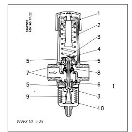
The valve plate (8) is a brass plate with a vulcanized layer of special rubber to form an elastic seal against the valve seat. The valve is externally sealed by the diaphragms (7).
