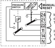
Manual reset timer contacts. Terminal 21 to 22 closed during normal run and during time-out – open on time-out. Terminals 21/24 (signal) closed after time-out.
