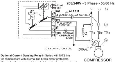
for compressors with internal line break motor protectors. (Prevents oil pressure safety control from tripping when internal line-break motor protector trips.)
