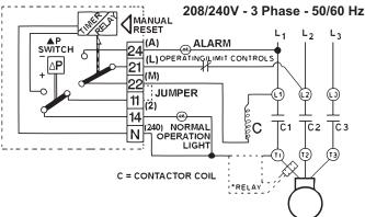
\* Optional Current Sensing Relay in Series with N/T1 line for compressors with internal line break motor protectors. (Prevents oil pressure safety control from tripping when internal line-break motor protector trips.)
