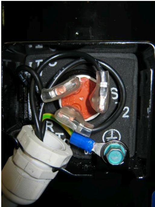
Figure 7: Correct electrical installation with cable glands for IP21 T-box (models ZS09KAE to ZS13KAE)
